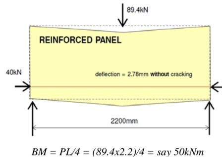
The post-tensioned panel deflected nearly 3mm without any visible signs of cracking.
