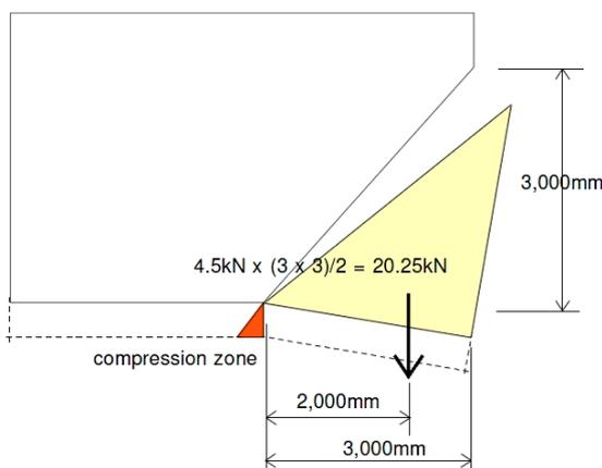
BM generated by rotation of brick panel =  $20.25\text{kN} \times 2\text{mtrs} = \text{say } 40\text{kNm}$ .
