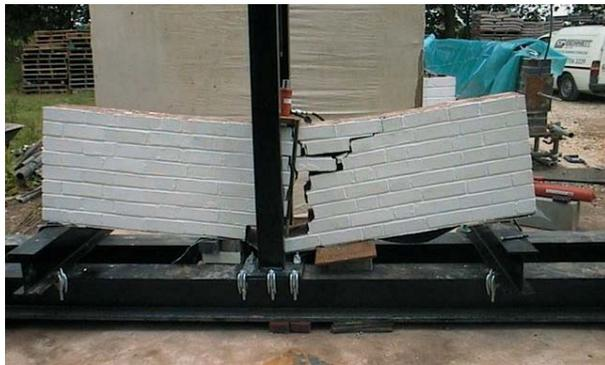
The panel was acting as a shallow truss with masonry in compression and the lower section of the panel in tension, as below.
